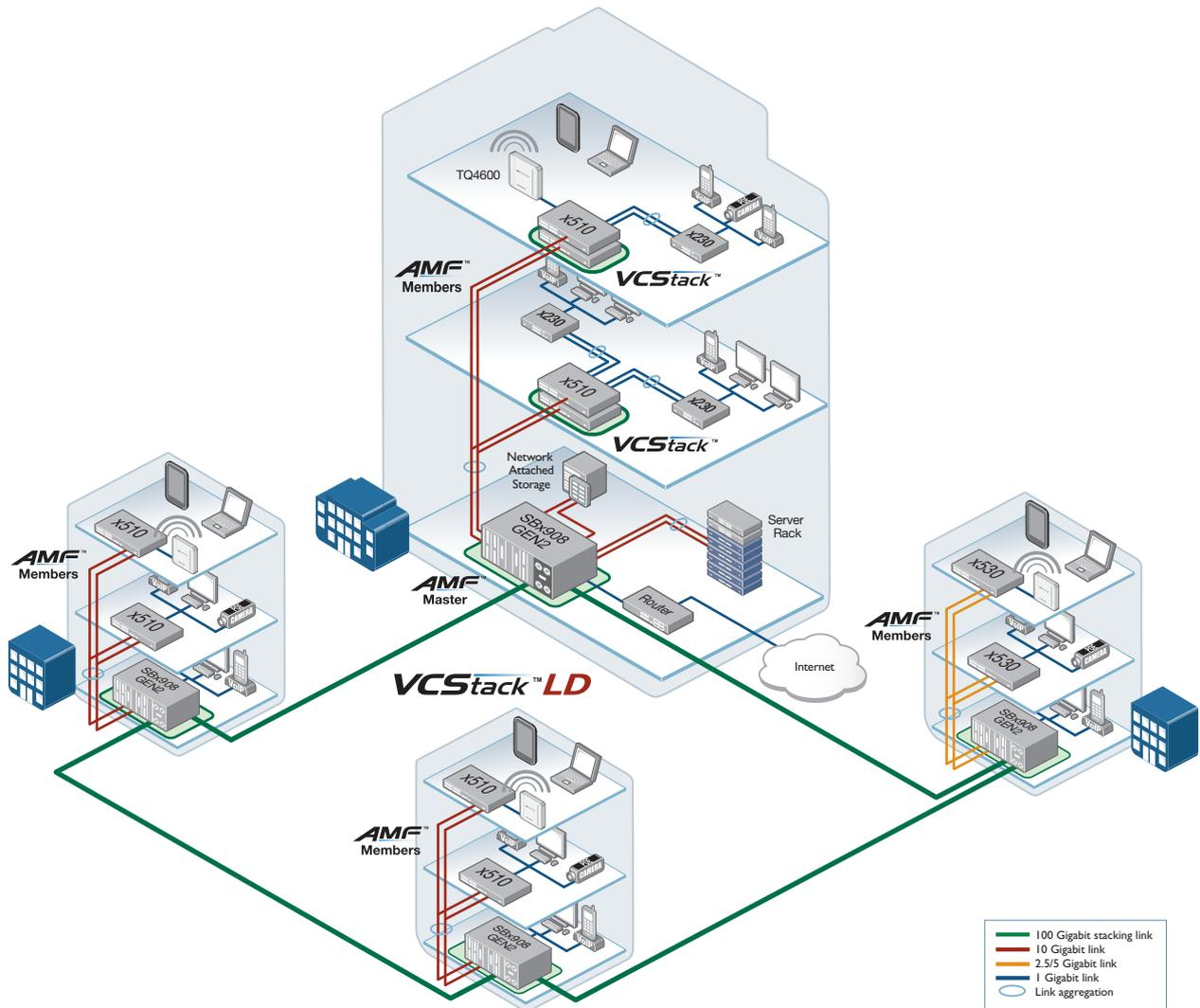
Today's large enterprises demand ready access to online resources and applications, and require a high-performing network that can seamlessly carry multiple converged services. This campus solution uses the SwitchBlade x908 GEN2 and long-distance Virtual Chassis Stacking (VCStack LD)—ideal for a distributed network core that provides high availability, increased capacity and ease of management.
