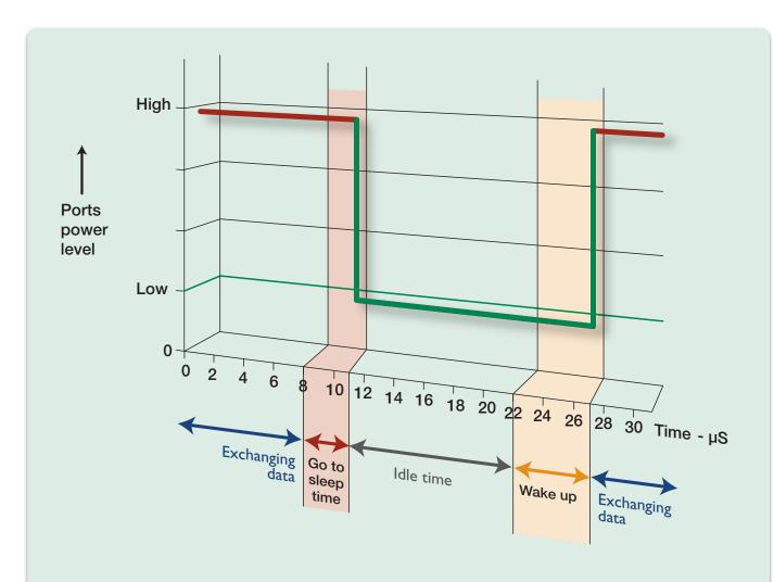
A compelling feature of EEE is its ability to take advantage of even very brief idle periods. An EEE port will move to low-power mode within just a few micro-seconds of no data. On a 10Gigabit port, the port can be down to low power in about 3 micro-seconds after sending a packet. So, power is not saved just in the long idle periods, but in all the thousands of brief idle periods that occur even when a workstation is active.
