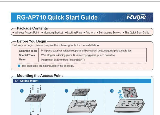
Step1: To fix the bracket to the ceiling, first tap the wall anchors into the holes, align the holes on the mounting bracket to the wall anchors, then drive the screws through the bracket into the anchors. **Step2:** Align the square feet on the rear of the access point over the mounting holes on the bracket. Step3: Slide the access point onto the bracket in the reverse direction of the arrow printed on the mounting bracket until it clicks into place.
